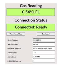
Axiom Diagnostic Tool (ADT) requires USB-C to USB PC cable connection. Axiom diagnostic information is available through a PC application, providing real time gas reading, access to configuration settings (baud rate, Modbus address) and detailed fault information to assist with service and maintenance.
