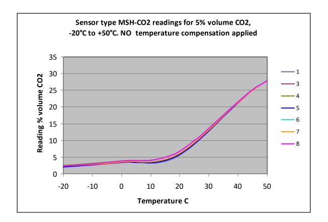
The non-linear nature of the span temperature dependency needs to be taken into account when applying temperature compensation. Whilst the variation from sensor to sensor is very small, multiple-point temperature compensations are required in order to achieve accurate results across the full operating temperature range.
