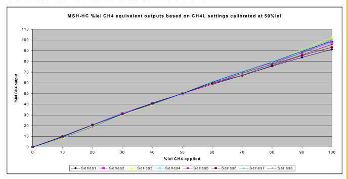
It is therefore recommended that the critical alarm point or full scale be the best calibration concentrations to select, depending on the application.
