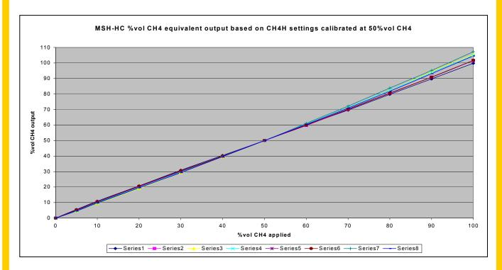
So again, the calibration point can be selected to optimise the accuracy at an appropriate level dependent on the application. Fine tuning of linearity coefficients can accommodate the linearity deviations but to enable a simple two point calibration (zero and span) it is more efficient to maintain default linearity coefficients and accept a small amount of nonlinearity.
