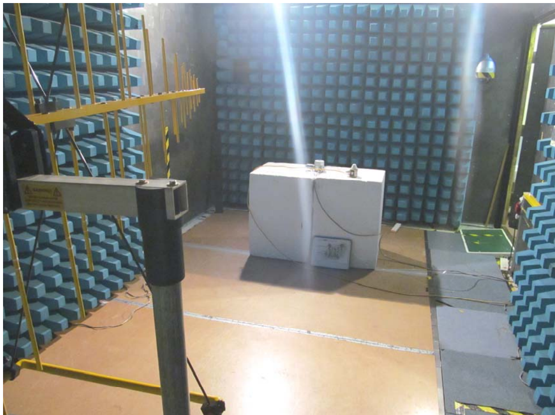
Photograph 5.4.2 Radiated immunity testing
