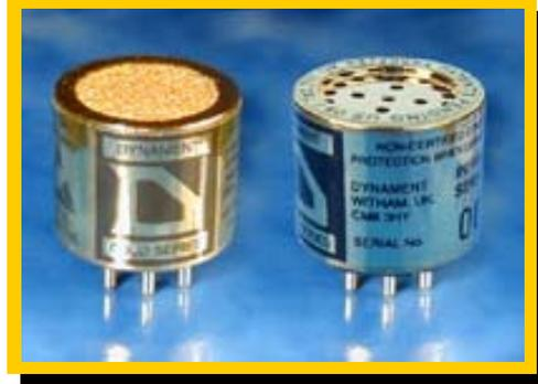
In order to derive a signal from the Dynament range of infrared sensors the lamp should be pulsed at a constant frequency and duty cycle and power should be applied to the on-chip FET transistors. The signal can then be extracted from the on-chip FET transistor sources and the internal sensor temperature can also be monitored continuously. A schematic of the sensor along with a pin-out diagram is shown below to assist in this discussion.
